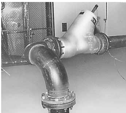
Figure 9 Size 10 Class 1500 Flite-Flow® inclined bonnet piston lift check valve with two upstream elbows. Test loop capacity permitted tests with line velocity over 20 ft/s (6 m/s).
